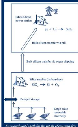
Envisaged supply path for the supply of emission-free silicon fuel for power generation
